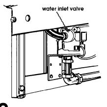
Connect water pipe or tubing directly to water inlet valve. Do Not run pipe or tubing across front of motor or dishwasher legs. Turn on water supply and check for leaks.
